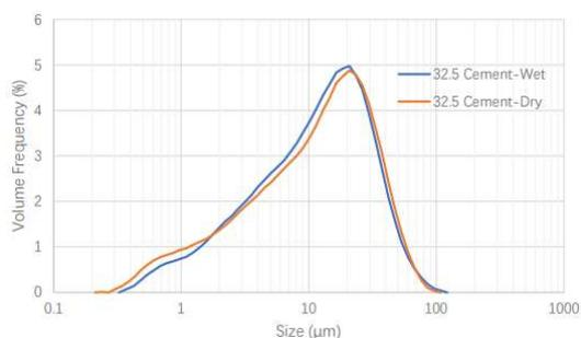
**Figure 2.** Particle size results of 32.5 cement by wet and dry dispersion
